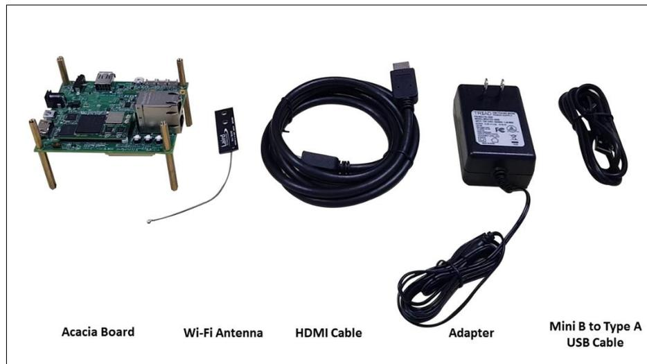
**Figure 3: Components of eSOMiMX7 Evaluation Kit**
